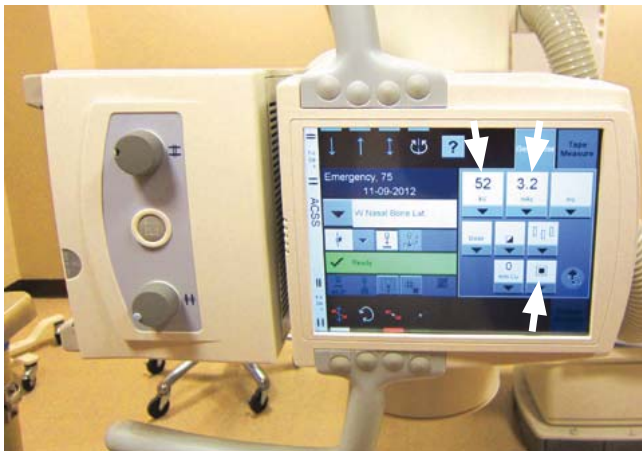
Figure 4. X-ray tube head demonstrating digital display of nasal bone exposure factors: 52 kVp, 3.2 mAs, small focal spot.
