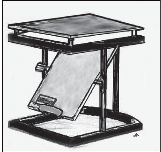
Fig. 3. Carpal Box apparatus. This box allows the radiographer to take an elongated or widened image of the wrist.
