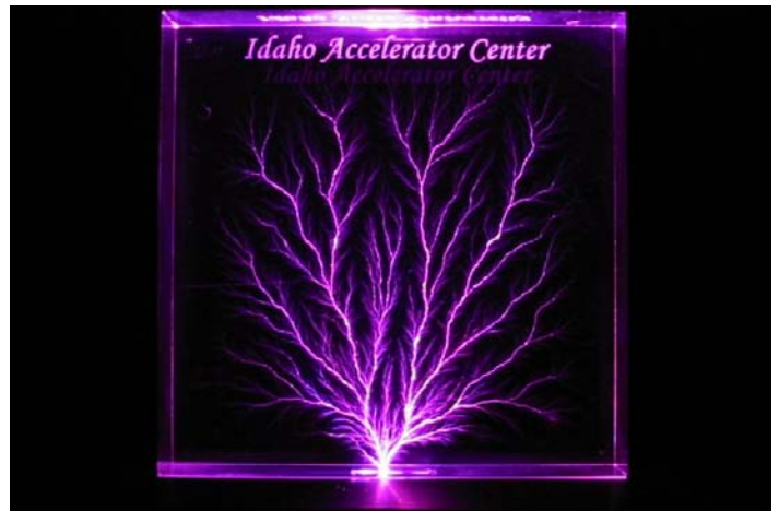
A “spark tree” produced by a rapid electrical discharge in plastic.
