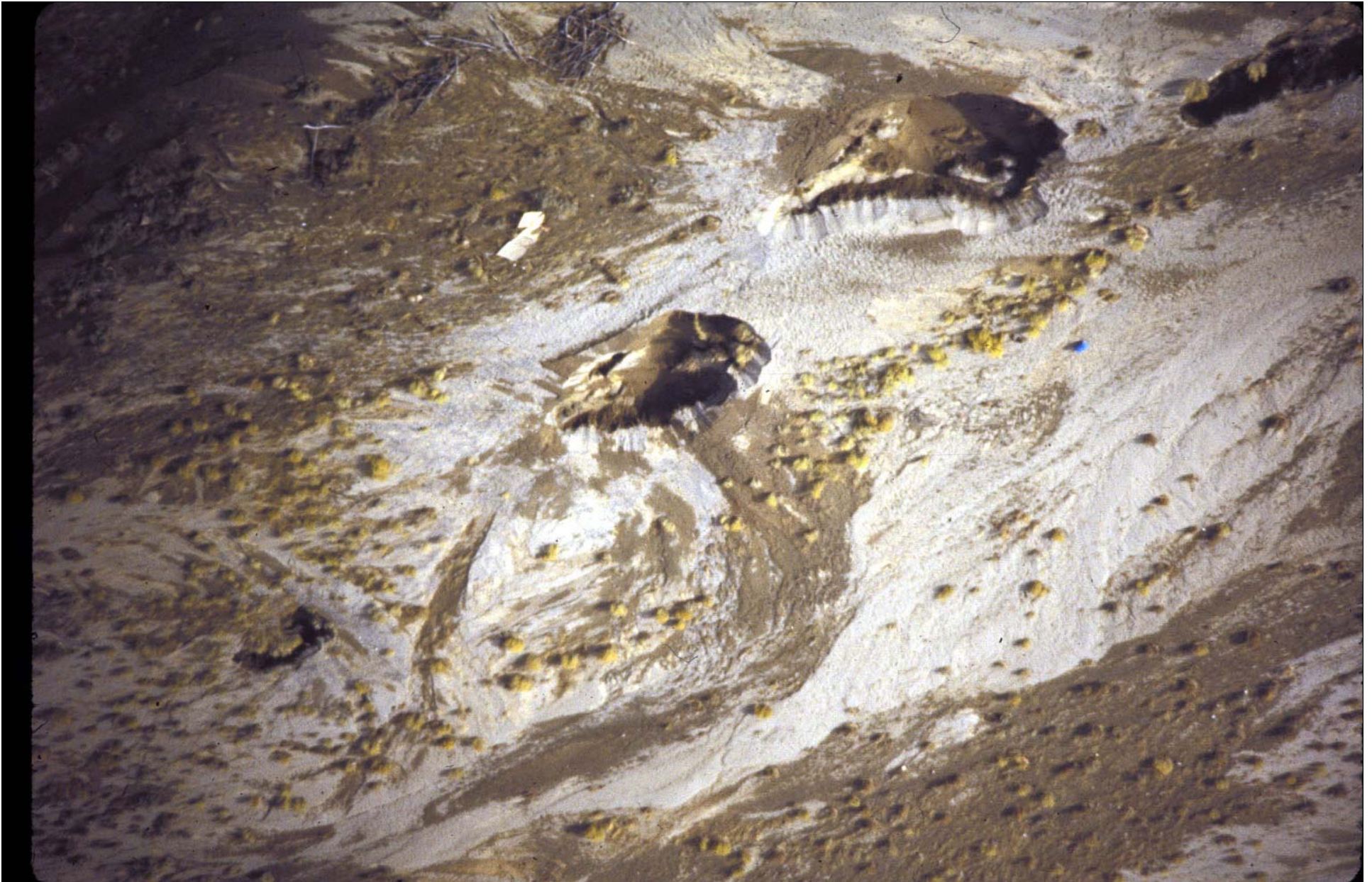
Sand Boils at Chilly Butte after the earthquake. Note small structures between the explosion craters.
